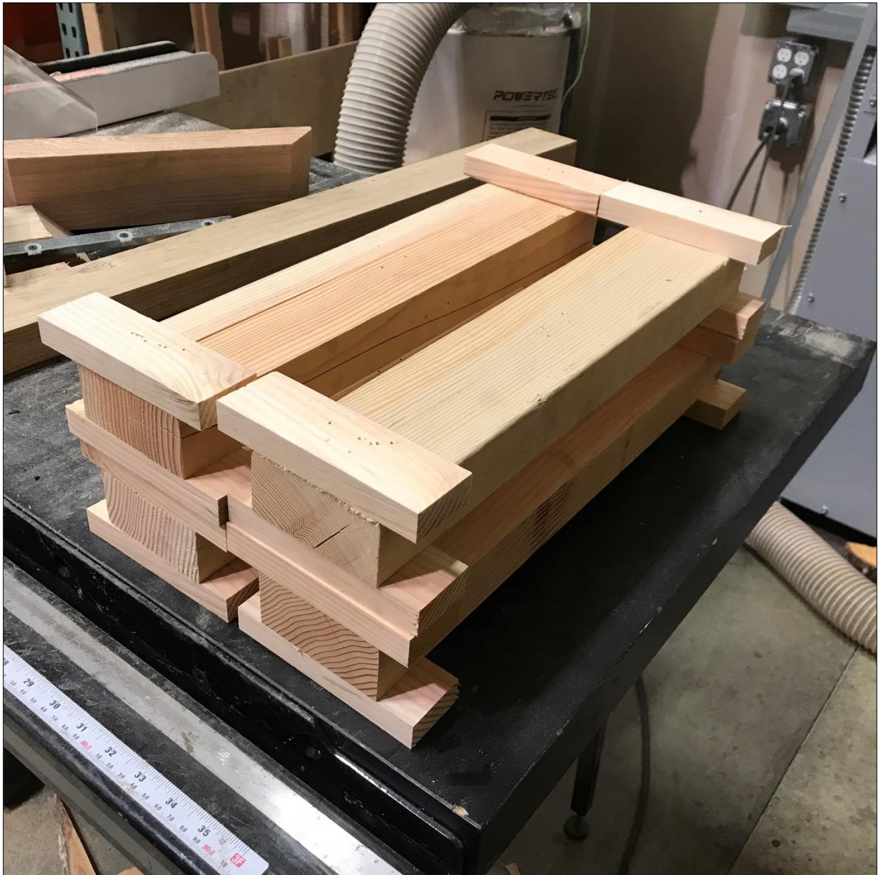
Typical Fuel Load
