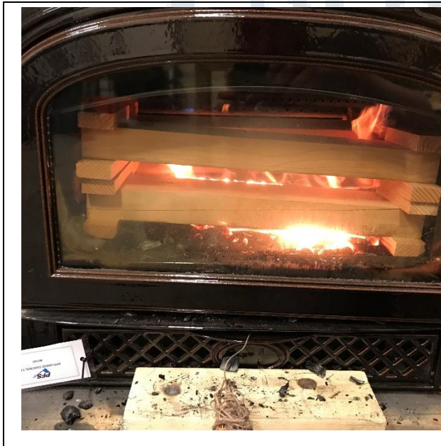
Test Fuel Loaded in Stove
