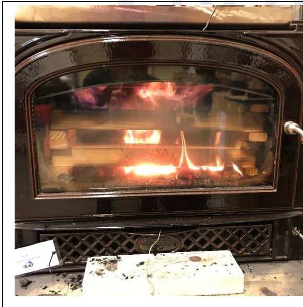
Test Fuel Loaded in Stove
