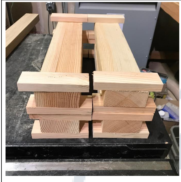
Test Fuel Side View
